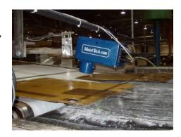
In board plants, the sensor is often installed in extreme heat locations typically near a pre-heater. In these situations, the gauge is fitted with a built-in Vortex Air Cooling System to optimize performance and extend the life of the instrument. Furthermore, the environment in board plants can be very moist so IR3000 comes standard with an air-diffuser nozzle which prevents condensation from collecting on the sensor's optical window.
